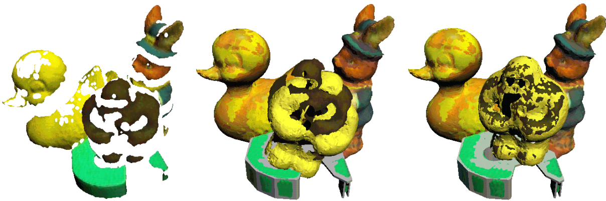
Figure 6.5 Scene view with missing data, roughly placed model and automatic matched model
