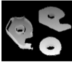
Figure 4.21 Range image of BIRIS scanner
