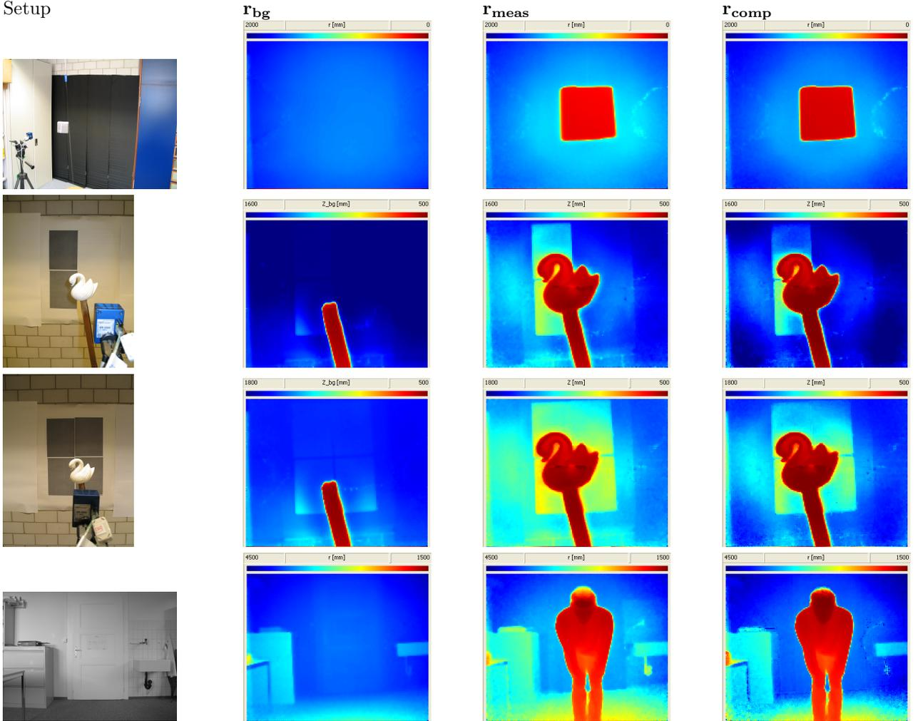
**Figure 5.** Scattering compensation experiments.  $\mathbf{r}_{bg}$  is the background range image,  $\mathbf{r}_{meas}$  is the measured foreground range image, and  $\mathbf{r}_{comp}$  is the foreground range image after scattering compensation.
