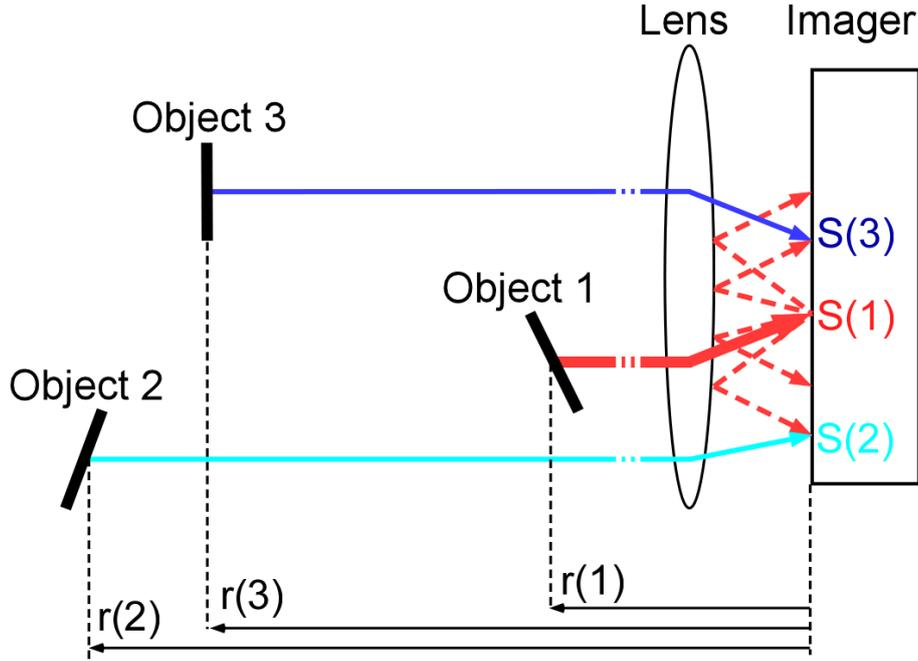
Figure 2. Light scattering in TOF camera .
