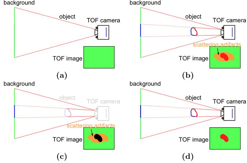
**Figure 3.** Experiment setup for scattering quantification. (a) : Background measurement  $\mathbf{r}_{bg}$ - (b) : Measurement with foreground object  $\mathbf{r}_{meas}$  - (c) : Background only image for foreground scene  $\mathbf{r}_{meas,masked}$  - (d) : Output with scattering compensation  $\mathbf{r}_{comp}$
